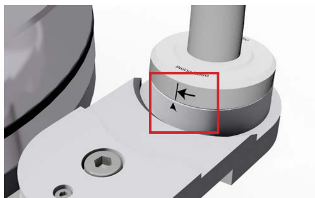
Pic 14b: Mounting direction of the upper part (to the right)
