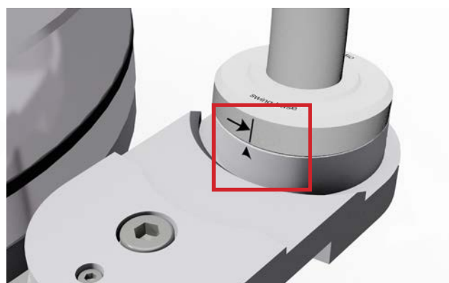
Pic 15b: Mounting direction of the upper part (to the rear)
